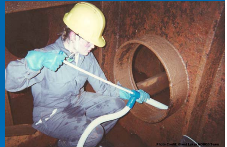
Pumping residual water with a hand-operated pump in a double bottom ballast tank.
