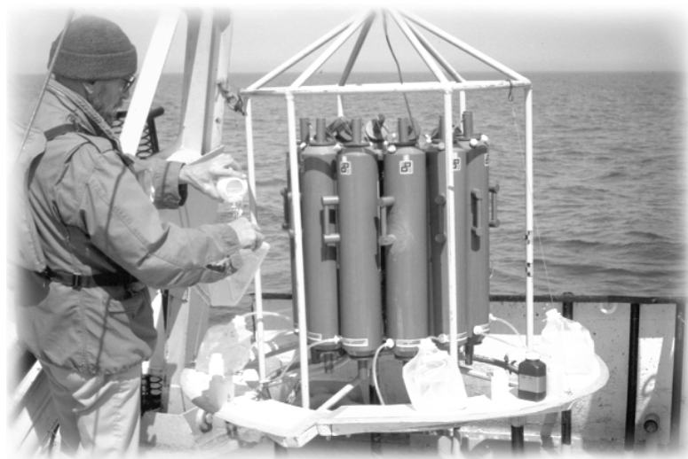
Sediment sampling aboard EPA research vessel, "Mudpuppy", Indiana Harbor Canal, East Chicago, IN. Photograph courtesy of the USEPA, ARCS program.
