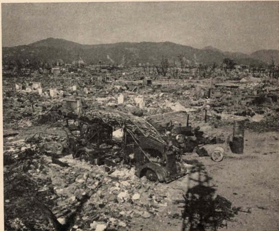
THE HIROSHIMA FIRE DEPARTMENT lost its only aerial ladder truck when the west side main fire station was destroyed by blast and fire, 4,000 feet from ground zero (Japanese photo).
