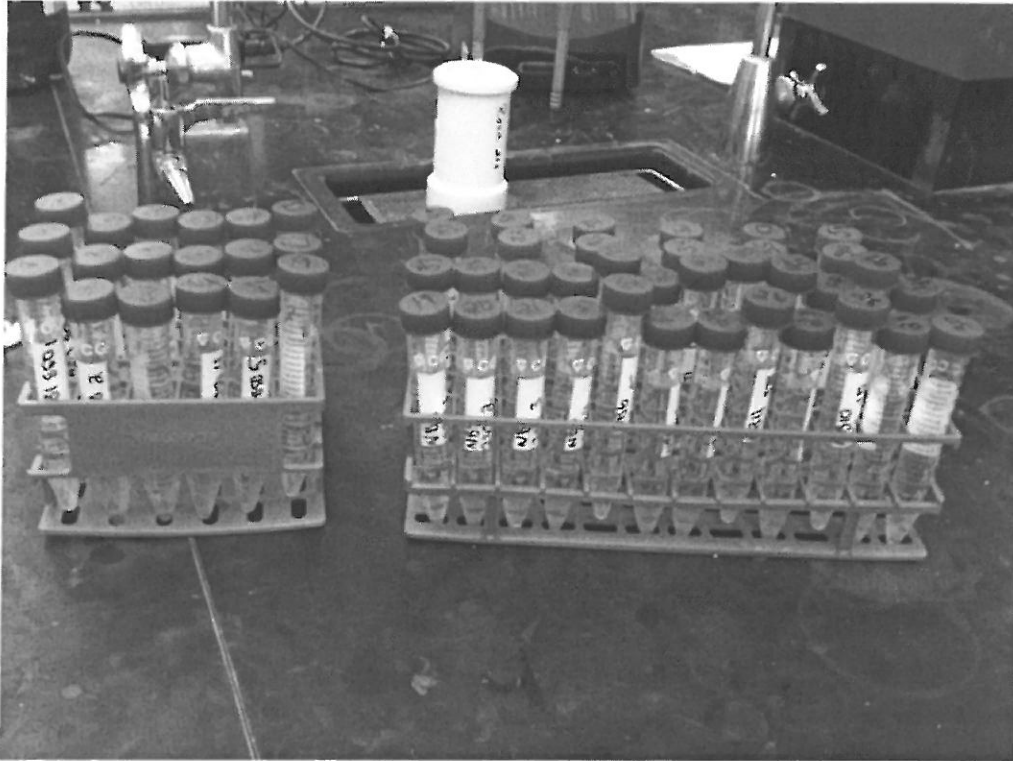
Figure 6. Image showing the 54 sample tubes prepared to be sent to URI for further analysis using ICP-MS.
