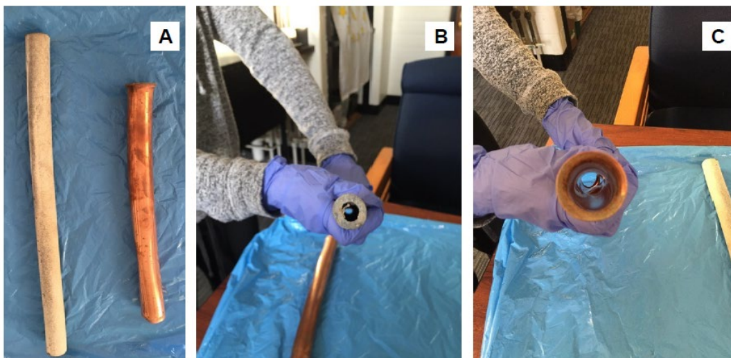
206 207 Figure 3: A comparison of old and new service lines (A); old lead line (B) and the new 208 copper line (C)
