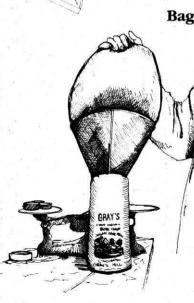
Bagging Room: Bags of justground flour are hauled into the bagging room, where it is scooped onto a scale, then poured through a funnel and bagged by hand. The tops of the bags are then pleated and fastened with the traditional miller's knot. **Sluice Gate Wheel:** This is used to open and close the sluice gate, which starts and stops the flow of water from the millpond across the street providing power to the water wheel to grind the grain. This dates back to 1740 when water was rushing
