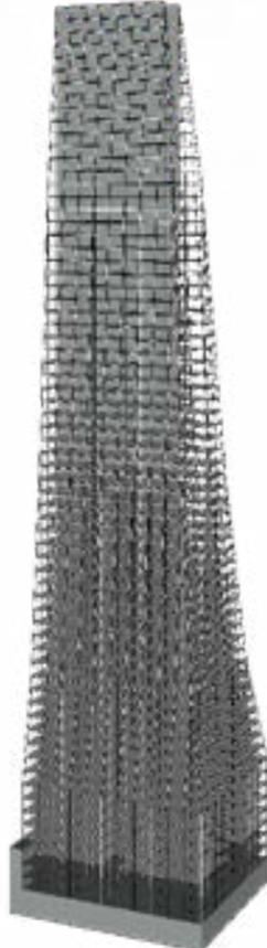
Timber Frame: structural system, floor plates and concrete pads (CLT and NLT combination)
