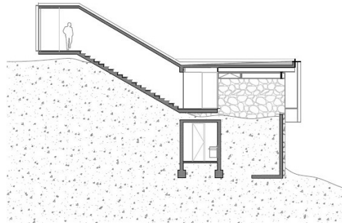
SECTION THROUGH STAIRCASE
